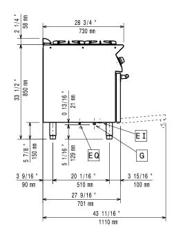
Electrical inlet (power) Gas connection
